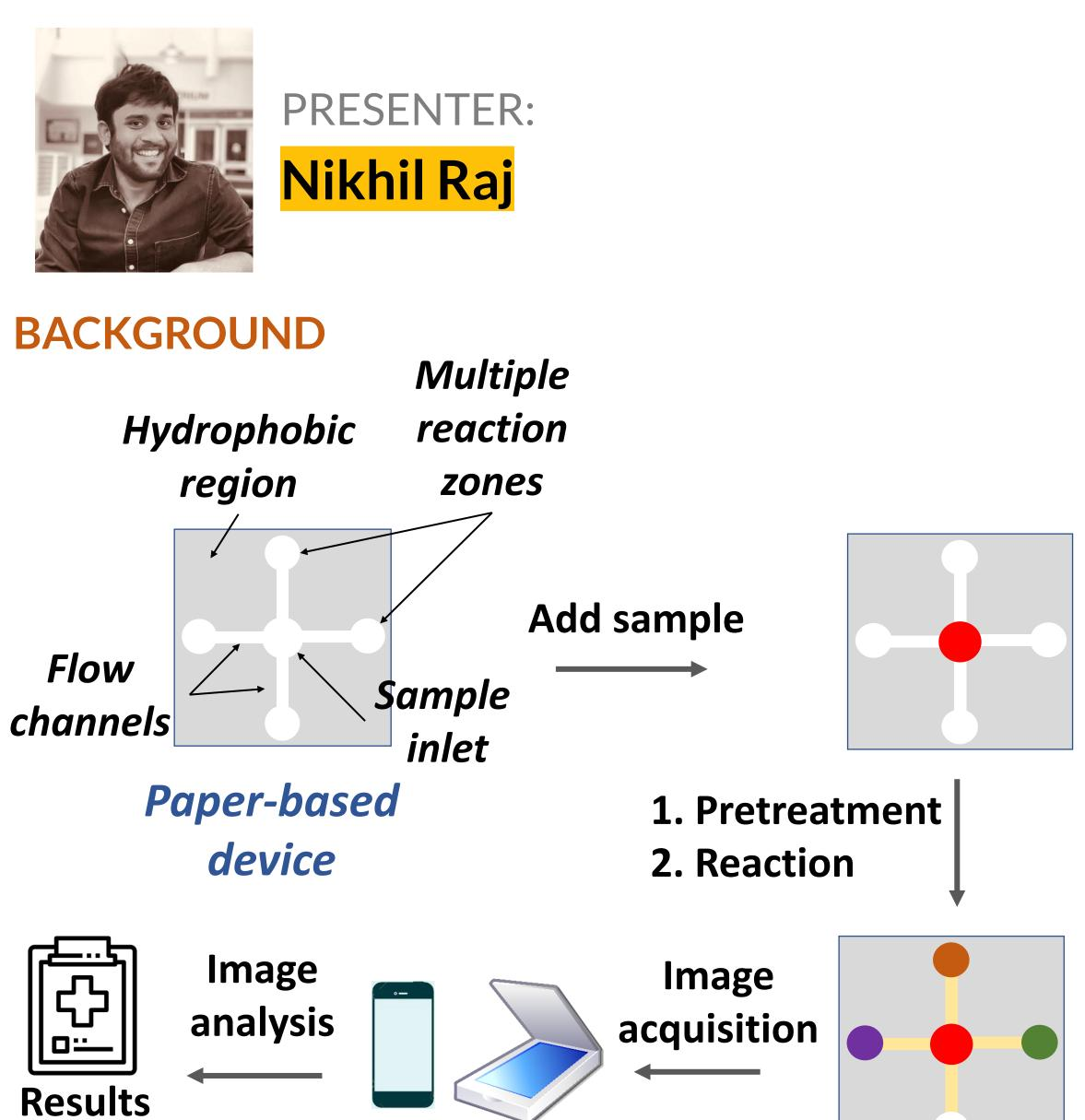
Sample testing procedure using paper-based sensors
